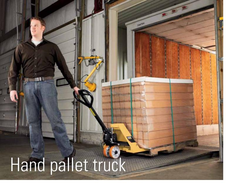
The hand pallet truck is without any doubt the most basic, yet essential, tool in materials handling.
